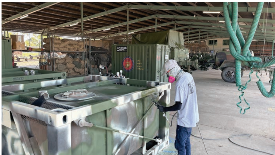
CST Technicians deployed to Darwin, Australia, to conduct intermediate level corrosion repairs using the CPAC MSC. (Photo by NSWCCD.)
